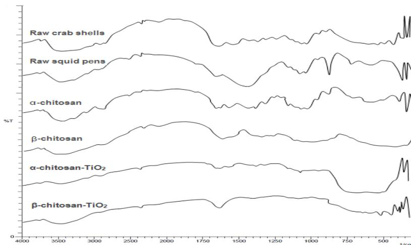
**Figure 1.** FT-IR spectra of crab shells, squid pens, chitosan and nanoparticle chitosan-TiO<sub>2</sub>.
