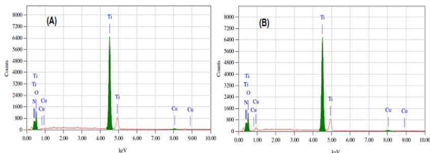
**Figure 2.** Data analysis of Energy Dispersive X-ray of (a) nanocomposite of  $\alpha$ -chitosan-TiO<sub>2</sub> from crab shells (b) nanocomposite of  $\beta$ -chitosan-TiO<sub>2</sub> from squid pens.
