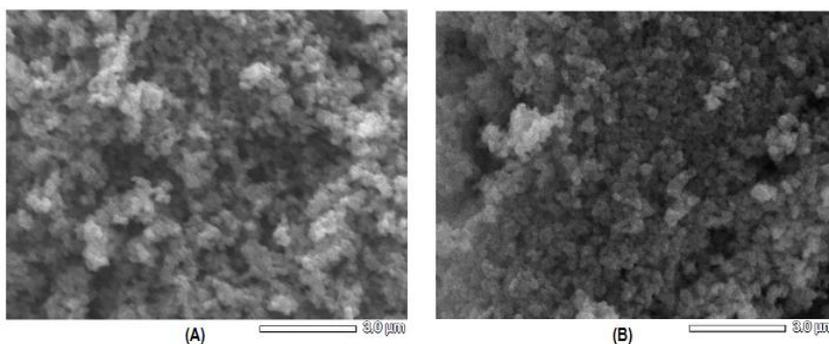
**Figure 3.** Scanning Electron Microscope (SEM) with magnification x10.000 for (a) nanocomposite  $\alpha$ -chitosan-TiO<sub>2</sub> from crab shells (b) nanocomposite  $\beta$ -chitosan-TiO<sub>2</sub> from squid pens.
