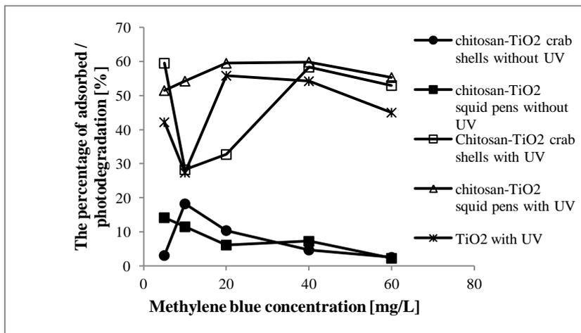
**Figure 4.** The concentration vs percentage of photodegradation of methylene blue by nanocomposite chitosan-TiO<sub>2</sub> and TiO<sub>2</sub> with and without UV irradiation.
